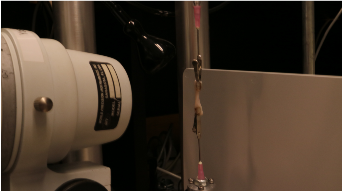
Fig. 3.5.: The fixture for tensile testing with a nerve fixed by alligator clips.
